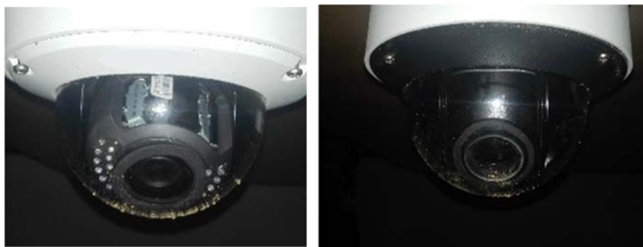
Figure 8 Dusty Environment Test
